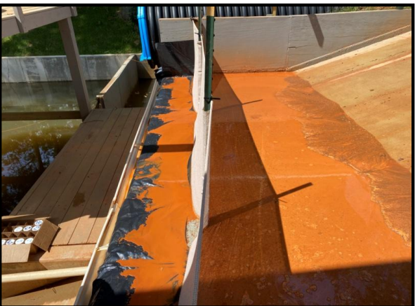
Ponding and Sediment Build-up Behind Product at end of Flow (30 minutes) and at end of Seepage (60 minutes)
