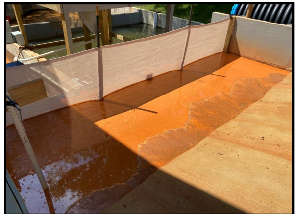
Ponding and Sediment Build-up Behind Product at end of Flow (30 minutes) and at end of Seepage (60 minutes)
